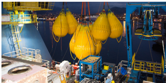
First large scale test completed by Water Weights using three 110T and four 55T bags manufactured by Structure-flex
