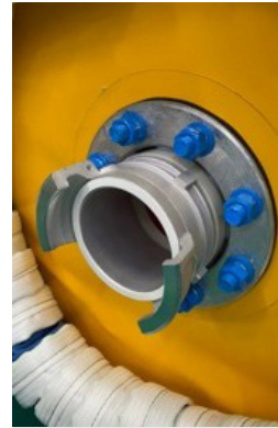
Bolted flange with 3 inch guillemin coupling
