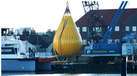
Prototype 110T bag undergoing initial trials in Great Yarmouth, UK
