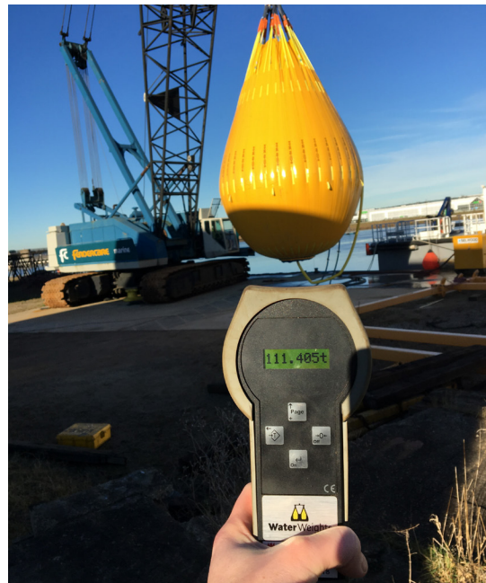
110T capacity easily and safely achieved on first prototype bag
